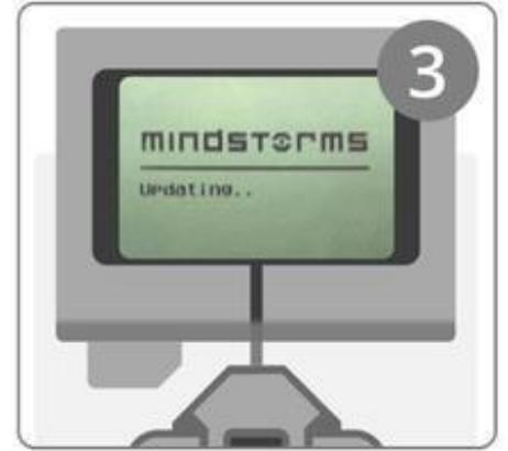
1. Hold down the Back, Center, and Right Buttons on the EV3 Brick.
